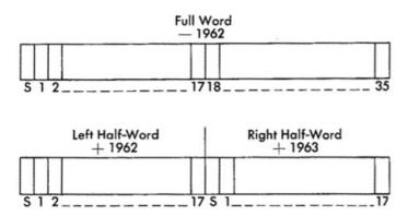
Most instructions use the sign bit of the instruction to indicate whether the address refers to a half-word, with a plus sign (sign bit of 0) or a full-word, with a minus sign (sign bit of 1).
